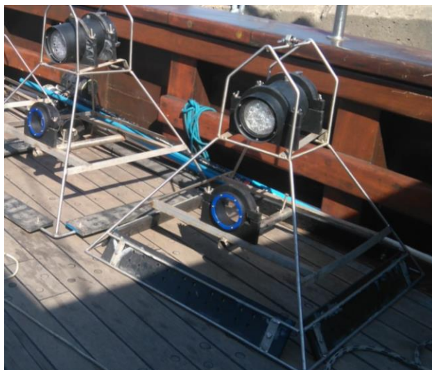
A mono-BRUVs frame with a light mounted on the top. ©Tamsyn Livingston, Ezemvelo KZN Wildlife.
